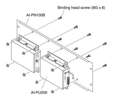
Step 2. Mount the AI-PN100B in a standard equipment rack.
